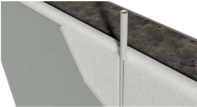
Services can be reticulated in the internal EPS panel.
